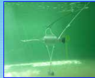
円周型魚眼カメラとその曳航試験 (A circular fish-eye lens and its towing test in water tank)
