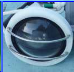
円周型魚眼カメラとその曳航試験 (A circular fish-eye lens and its towing test in water tank)
